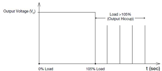
Additionally, if the  $I_o$  is  $< 130\%$  but  $> 110\%$  for a prolonged period of time (depending on the load), the Over Temperature Protection (OTP) will be activated due to high temperature on critical components. The power supply will then go into hiccup mode until the fault is removed; and, the input voltage is removed, then reapplied.
