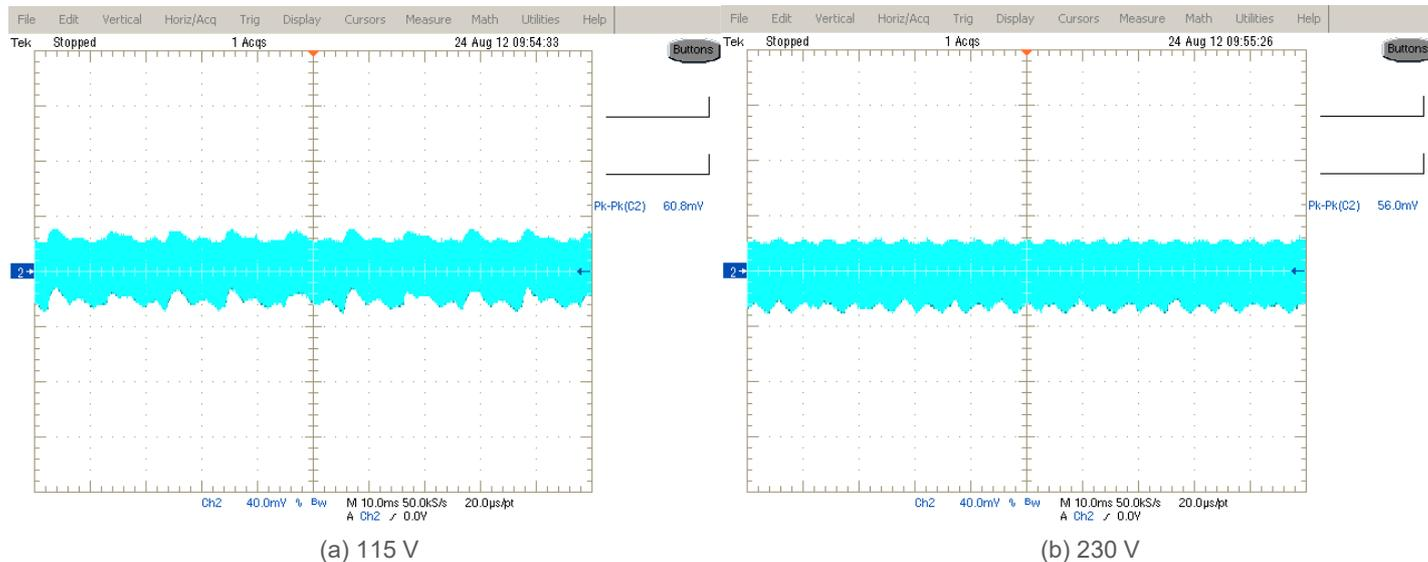
Fig. 2 Ripple & Noise example, 20 MHz BW
